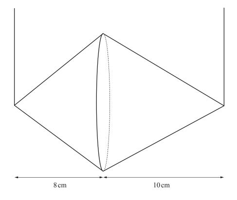
The object is suspended with a string attached to the vertex of the cone and another string attached to the vertex of the conical shell. The object is in equilibrium with the strings vertical and the axis of symmetry of the object horizontal (see diagram).
