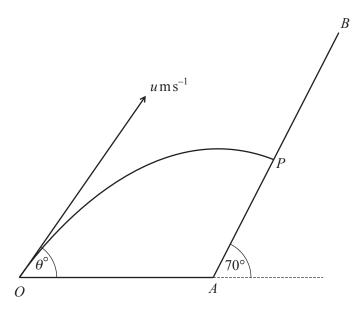
The diagram shows a surface consisting of a horizontal part OA and a plane AB inclined at an angle of 70° to the horizontal. A particle is projected from the point O with speed  $u \text{ ms}^{-1}$  at an angle of  $\theta^{\circ}$  above the horizontal OA. The particle hits the plane AB at the point P, with speed  $14 \text{ ms}^{-1}$  and at right angles to the plane, 1.4 s after projection.
